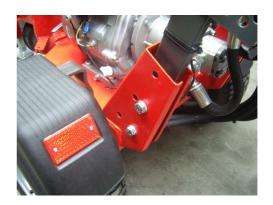
The second is on the upper part of the handles. Release M10 screws. Raise or lower the handle to a comfortable position and tighten screws.
